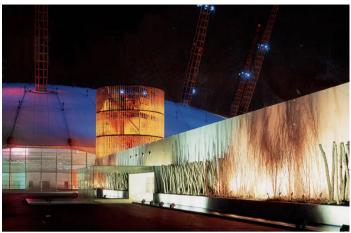
For the piazza, a grid of ground-recessed LED colour-change fittings blink and change colour on the hour, helping to orient visitors in both place and time. The Millennium Gardens were envisaged as a dark contemplative area, so we approached the lighting with a simple 'field of stars' on a 14m grid, bounded by the subtly illuminated Living Wall.
